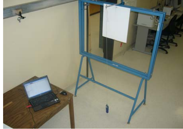
Figure 2. Experimental setup of the 3-axis accelerometer - altimeter as a simple pendulum.
