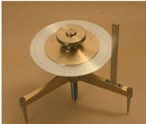
Figure 6. Grunow’s circa 1860 spherometer (Photo courtesy of Smithsonian Institution)
